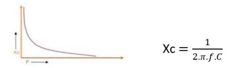
Presence of Harmonic distortion due to the non-linear loads within the network or due to import of harmonic from grid or power source will increases the current flowing through capacitors as the capacitive reactance is inversely proportional to the frequency, consequently capacitors will be subjected to overload. The overload on capacitors can cause premature failure in capacitor due to increased voltage and thermal stress on dielectric.
