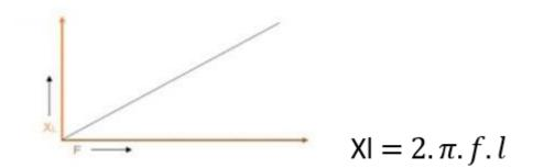
On the other hand, the inductive reactance XL of a Reactor is directly proportional to frequency: The magnitude of inductive reactance will increase with high frequency harmonics thus blocking the harmonic current. Hence, use of detuned reactor in series with capacitor will offer higher impedance for harmonics, thus eliminating risk of over load in capacitors.
